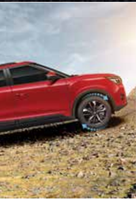
HILL HOLD ASSIST Hill hold assist technology prevents rolling back on an incline.
